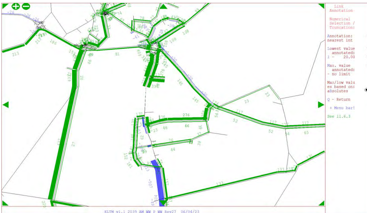
Figure 8 – 2039 WWGA Scenario 1: Traffic flow differences with and without 4,000 dwellings at WWGA: AM peak
