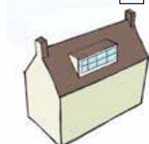
Loft conversion incorporating a long shed dormer which is out of scale with the original building.
