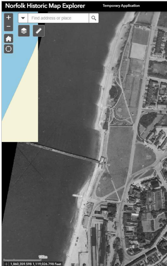
Figure A-17 Aerial photograph of the concrete groynes frontage. Exact date of the photograph is unknown, but taken between 1945-6 and 1960-1965. Crown Copyright, source: http://www.historic-maps.norfolk.gov.uk
