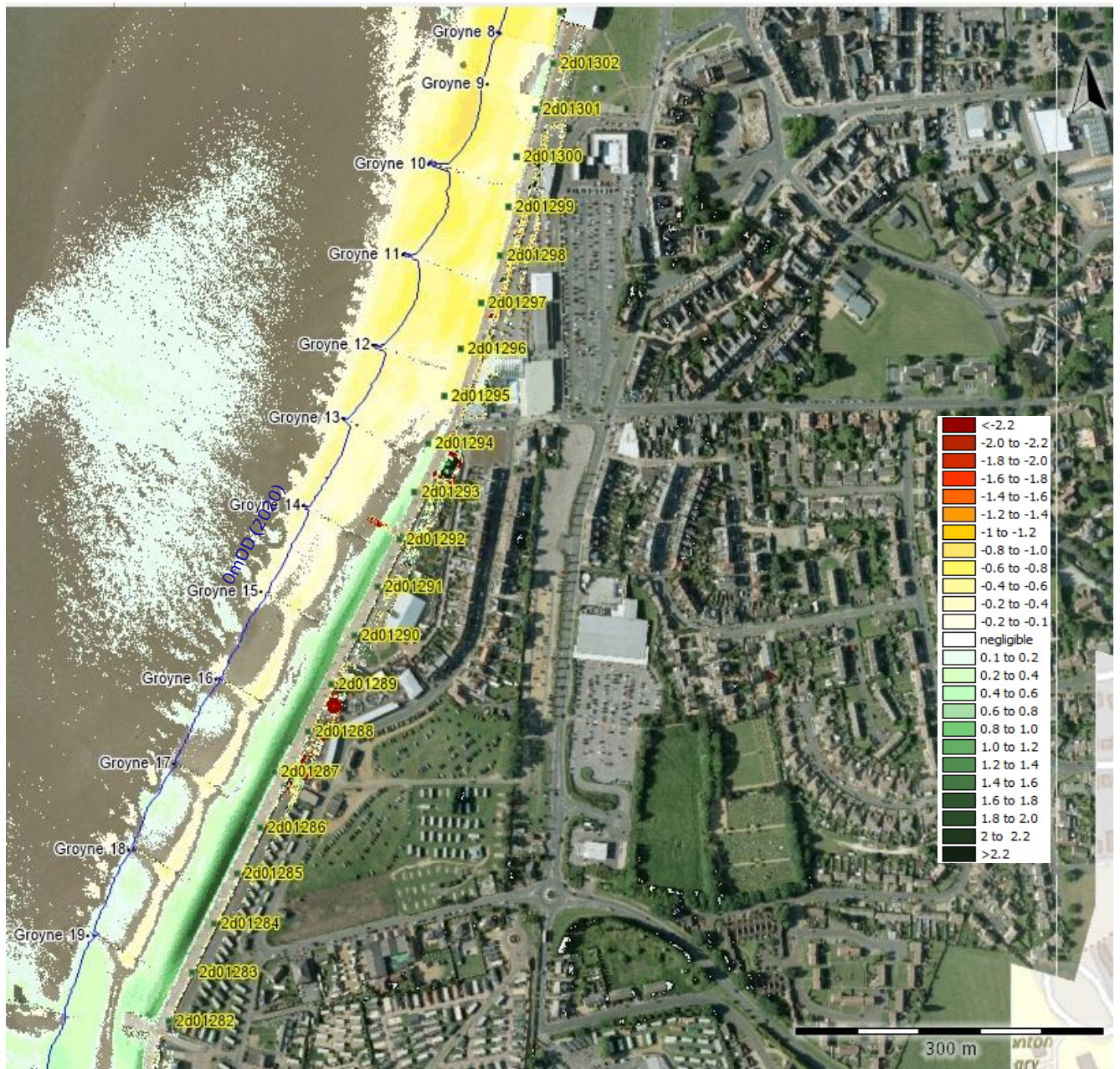
Figure A-31 Difference plot for the BCKLWN timber groyne frontage, generated from LiDAR data from 2020 and 2011, with change in beach level in m. (data courtesy of ACM). Negative values (green) mean that there has been a drop in level in 2020, and positive values (red and yellow) indicate an increase in level.
