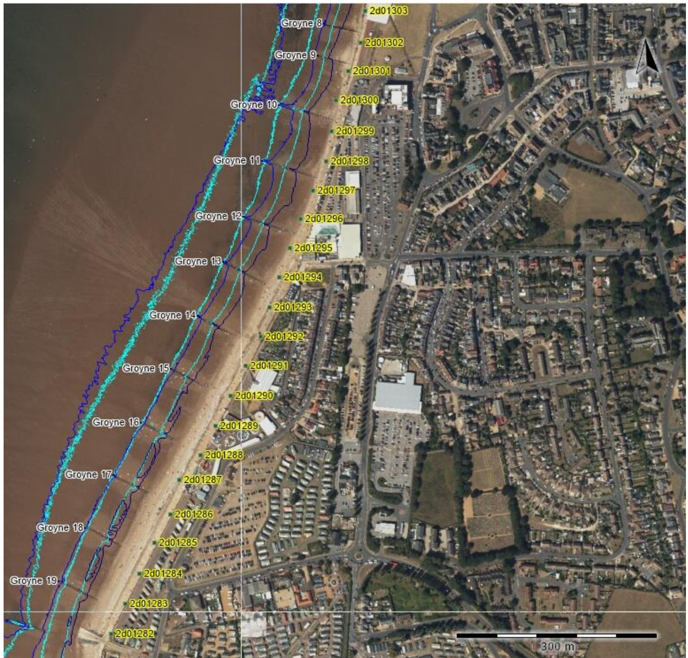
Figure A-32 BCKLWN timber groynes frontage, with the position of the +1 mOD, 0 mOD and -1 mOD contours generated from 2012 (light blue) and 2020 (blue) LiDAR data. Also shown are the beach transect locations. 2020 aerial image courtesy of ACM.
