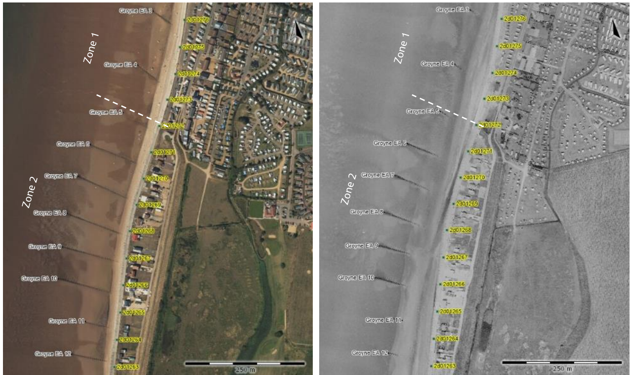
Figure A-39 Change in groyne exposure illustrating the change in the upper beach over time: left is 2020, right is 1992. Aerial images courtesy of ACM.
