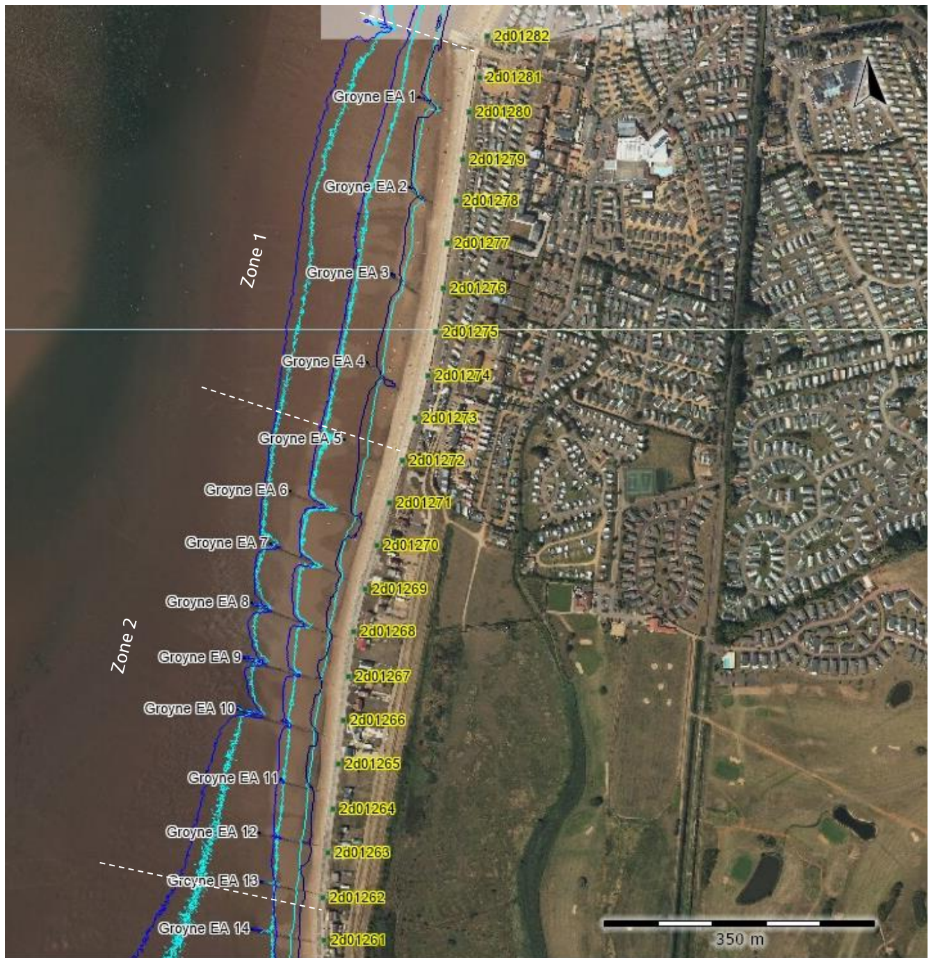
Figure A-44 Environment Agency timber groyne frontage Zones 1 and 2, with the position of the 0 mOD, +1 mOD and -1 mOD contours generated from 2012 (light blue) and 2020 (blue) LiDAR data. Also shown are the beach transect locations. 2020 aerial image courtesy of ACM.
