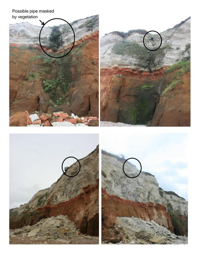
Surface staining is present along several sections of the face of the Carstone, which suggests that water does percolate out of the rock face, although being dry at the time, it is not known if this water originates as surface water flowing directly across the ground surface above and down the face, through joints in the chalk or along the interface between the chalk and the Carstone.
