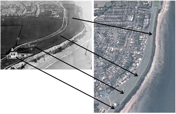
Currently, there are four visible fence lines or lines of fence posts along the cliff top, which are considered to have been erected as the cliff top progressively failed in order to keep the public a safe distance from the crumbling crest. Some concrete fence posts and wire are also present along the beach, which is also evidence of the progressive failure.
