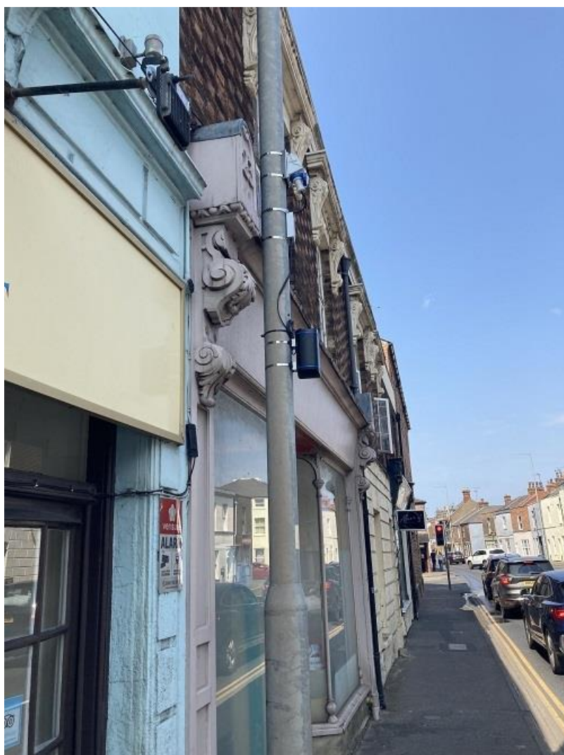
Figure C.1 – Earthsense Zephyr located along Railway Rd close to area with highest NO 2 concentrations.
